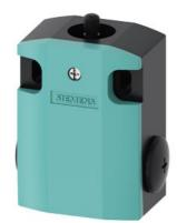
Basic switch for position switch 3SE51 Metal enclosure 56 mm Device connection 3x (M20x 1.5) 1 NO/1 NC quick action contacts without actuator head
