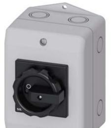
SENTRON, Switch disconnector 3LD, main switch, 3-pole, lu: 16 A, Operating power / at AC-23 A at 400 V: 7.5 kW, molded-plastic encapsulation for metric cable gland, rotary operating mechanism, black
